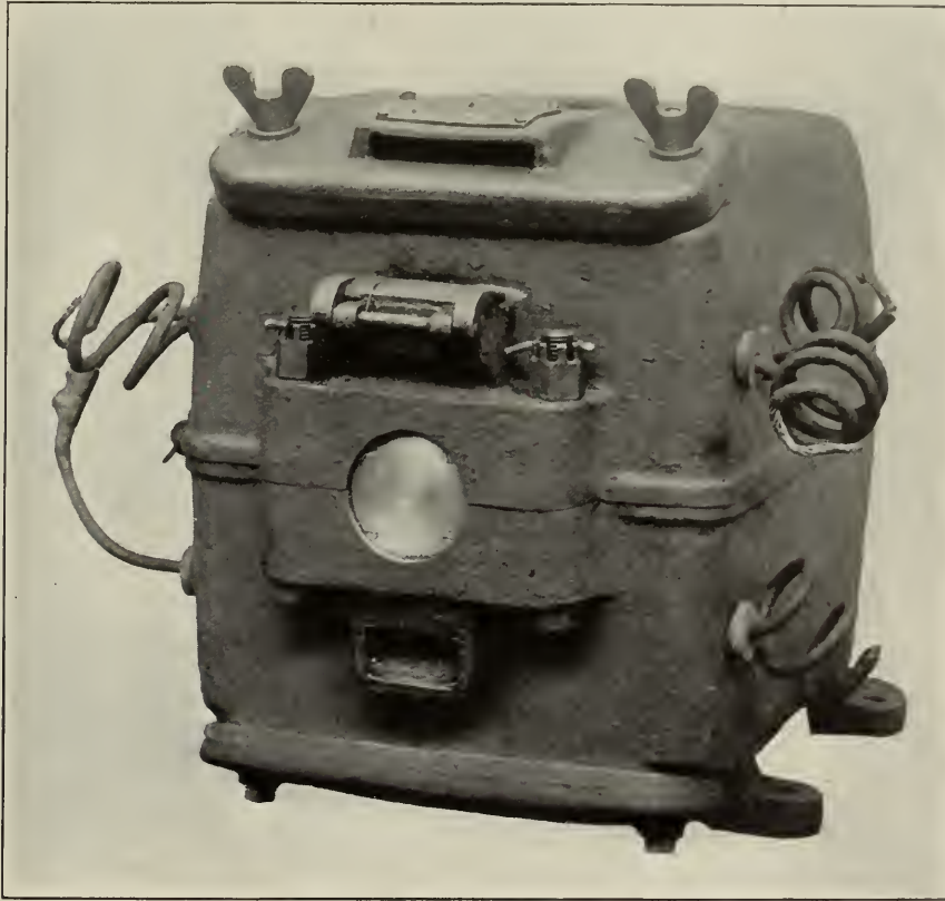
FIG. 2. HERMETICALLY SEALED MINING MOTOR. THE HELIOS COMPANY.
